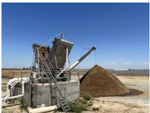
This machine separate manure into solids and liquids to be stored in a nearby anaerobic digester
