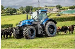
This prototype EV Tractor, the T7 Manure Power LNG uses methane from liquid manure as its power source!
